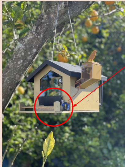
Micro servo motor + placement on The Smart Bird Feeder
